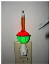
A **bubble light** is a decorative device consisting of a liquid-filled vial that is heated and lighted by an [incandescent light bulb](#). Because of the liquid's low [boiling point](#), the modest heat generated by the lamp causes the liquid to boil and [bubble](#) up from the vial's base thus creating a decorative effect.
